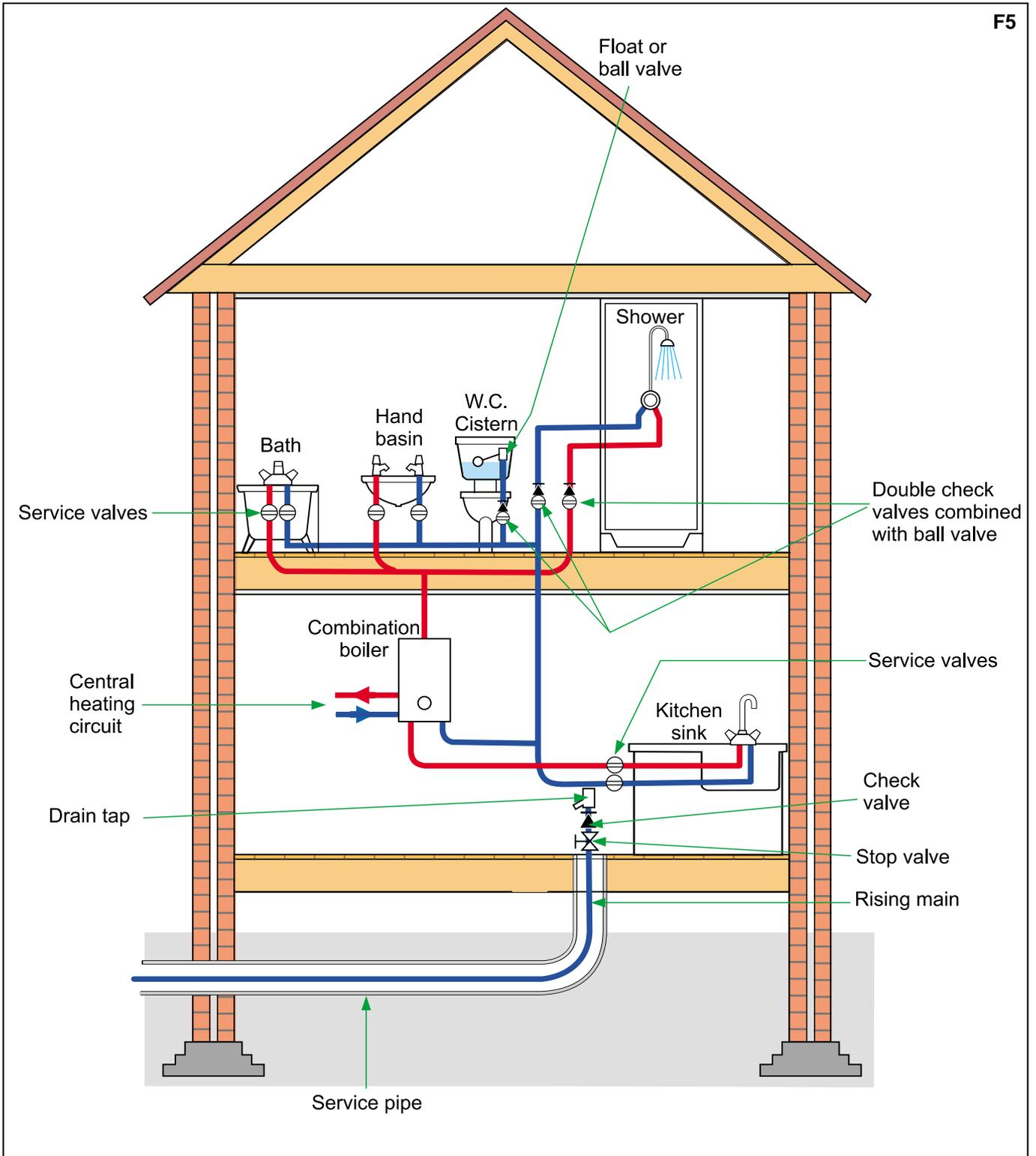
**A direct supply system** fitted with a modern boiler, anti-syphon and backflow devices (**F5**) complies with most modern water by-laws and eliminates the dangers of bacterial contamination.
