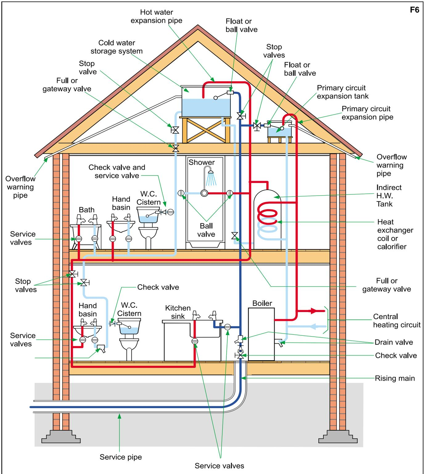
**An indirect system (F6)** supplies all sanitary appliances – hand basins, showers, baths and WCs – with water fed from a storage tank. Mains water, for drinking, is available at the kitchen tap only. This can also supply washing machines and a garden tap, which must be fitted with a check valve.
