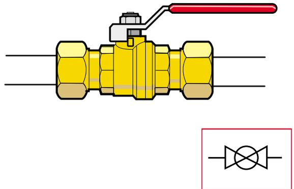
Service valves are available as straight (**F15**) and 90 degree bend (**F16**). They may be fitted into pipe-work adjacent to taps or may be specially designed for use with washing machines and dishwashers (**F17**). These valves restrict the water flow – unlike the ball valve, which is handle operated (**F18**) – only require a quarter turn and do not restrict the flow of water. They are ideal for use in conjunction with showers.
